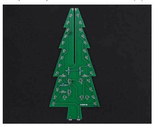
Step 2: Install 3pcs 4.7K Metal Film Resistor on R1,R3,R5
