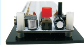
Then load the top transparent panel and lock with a shorter screw
