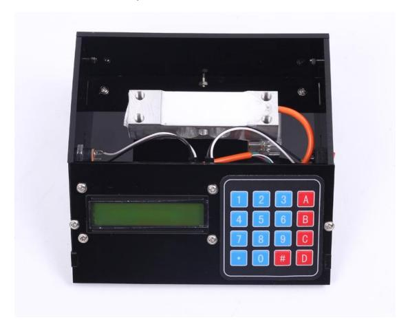
Step 19: Install Load-bearing acrylic with 4pcs Acrylic Gasket by M7\*30 screw fixed.
