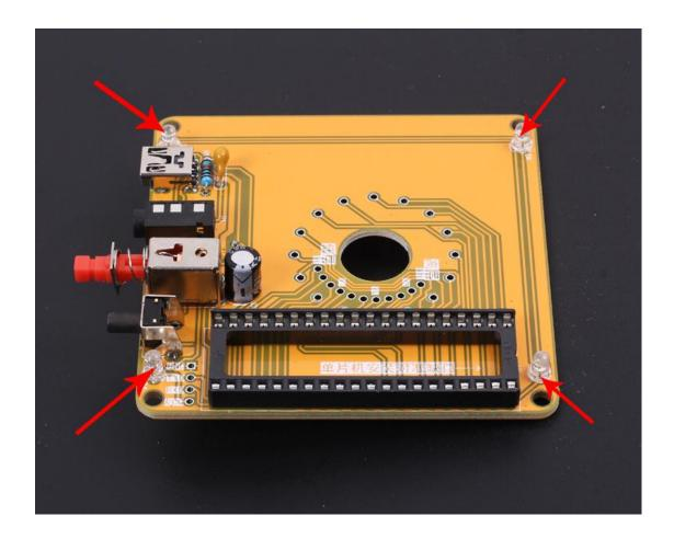
Step 6: Install Copper Pillar and Screw.
