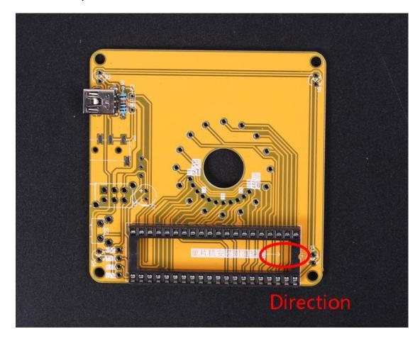
Step 2: Install 1pcs Monolithic Capacitor and Audio Socket.(User can install 4pcs 3mm LED work indicator on D1-D4 in this step and Note the direction.)
