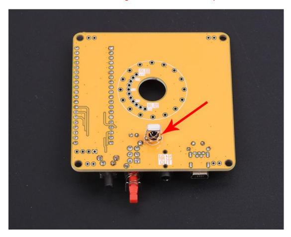
Step 5: Install 4pcs LED work indicator on D1-D4 and Pay attention to the installation direction.(If your have install LED on step 2,Please ignore Step 5 in here)
