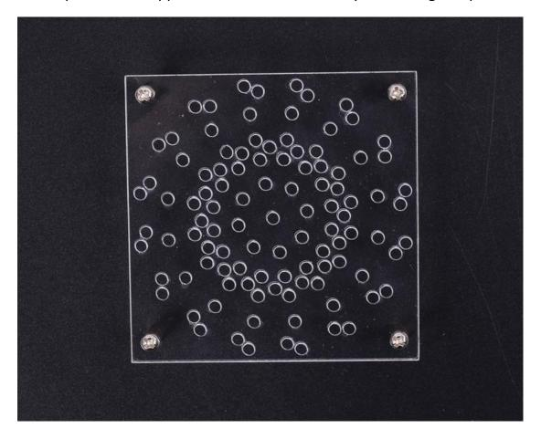
Step 8: Acrylic Welding Template Ring,LED Layer and Anode solder pad corresponding relationship.
