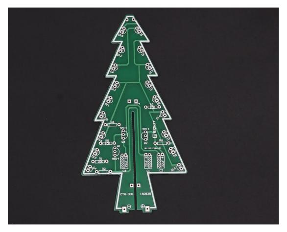
Step 8: Install 1pcs Metal Film Resistor 330ohm on R6, 1pcs 1K on R4, 1pcs 2K on R2
