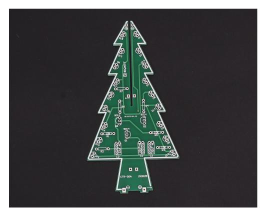
Step 1: Install 1pcs Metal Film Resistor 330ohm on R6, 1pcs 1K on R4, 1pcs 2K on R2
