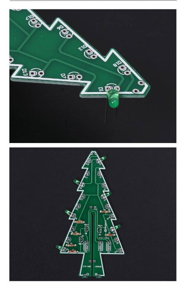
Step 11: Install 6pcs Red LED on D7-D12,6pcs Yellow LED on D13-D18
