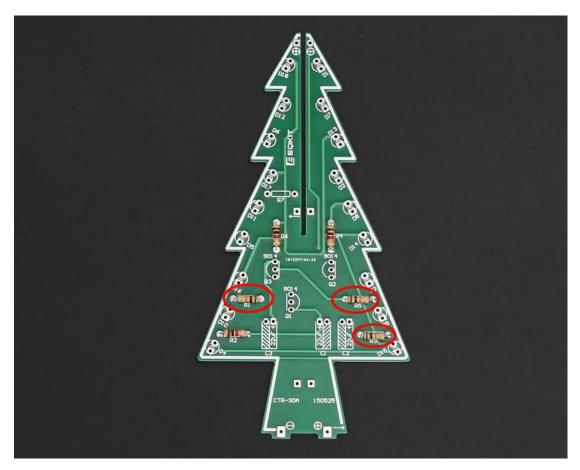
Step 2: Install 3pcs 10K Metal Film Resistor on R1,R3,R5
