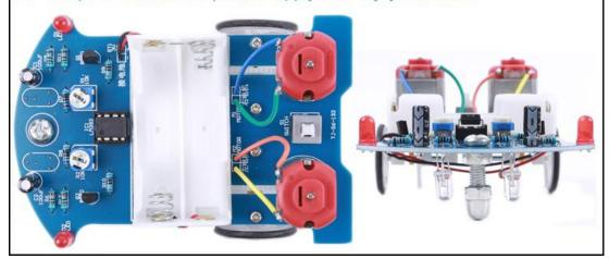
35>.Step 35: If the robot does not track the line very well, make small adjustments the to trimpots and then retest the line following. You can improve the ability of the car to follow the line by repeatedly testing and adjusting the pots by small amounts.
