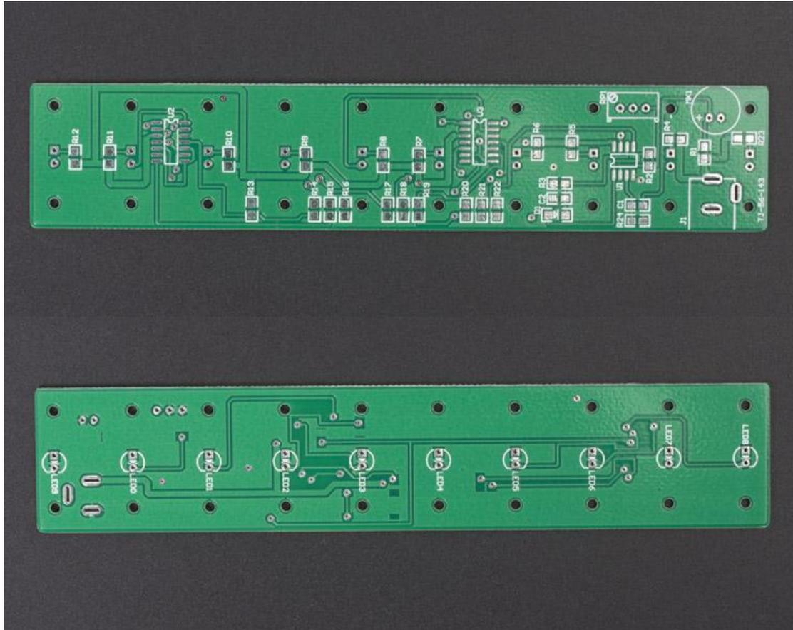
Step 1: Install 1pcs LM358 on U1 and 2pcs LM339 on U2,U3.Pay attention to the installation direction.
