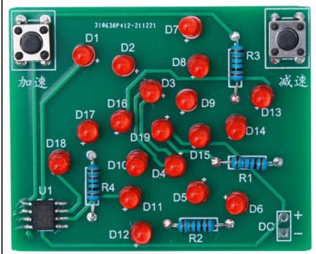
Step 7: Connect 5V work voltage and then press buttons to adjust display effect.
