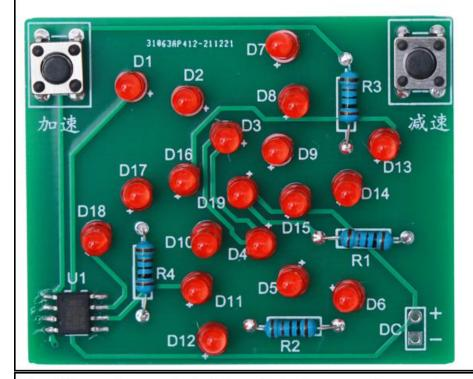
Step 6: Connect power pin by 2pin male pin.Users can also use other power sockets or directly connect the wires.
