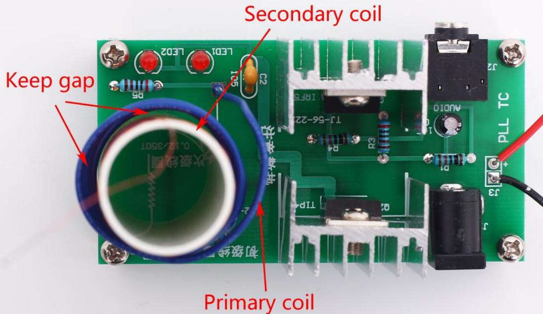
**Note:** There is no direct contact between the primary coil and the secondary coil, and the gap must be reserved, otherwise it may not work properly.
