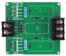
Step 6: Install 1pcs 3Pin HB950 Terminal at J2.
