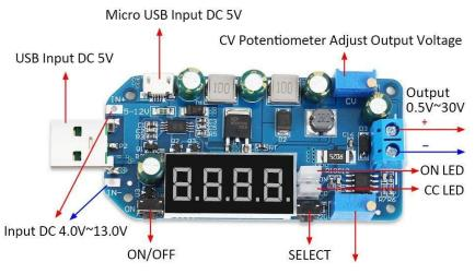
CC Potentiometer Adjust Output Current
