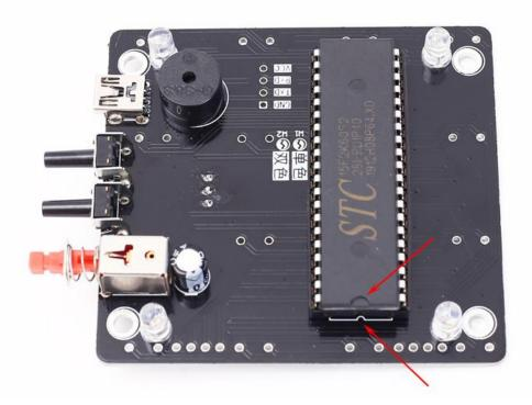
Step 10: Test.Connect work voltage by USB cable and MINI USB socket.Then turn ON red power supply switch.
