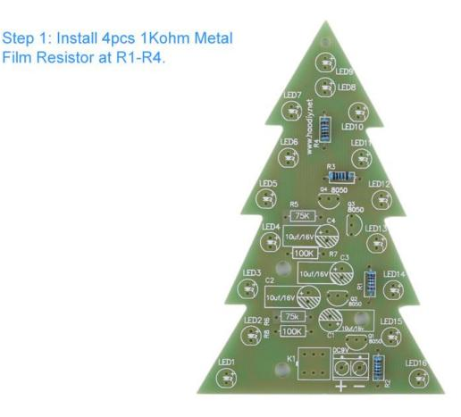
Step 2: Install 2pcs 75Kohm Metal Film Resistor at R5-R6.
