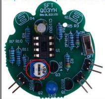
Step 14: Install 1pcs DIP-8 IC LM358P at U1. There is a groove on one end of the IC and there is a groove mark on PCB where the IC can place on. These two marks are corresponding to each other and are used to specify the installation direction of the IC.
