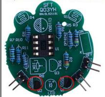
Step 9: Install 1pcs TO-92 S9014 Transistor at Q3.
