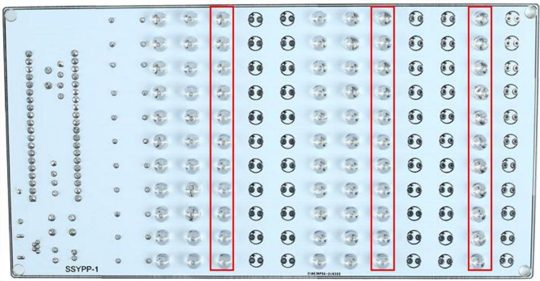
Step 15: Install 33pcs 5mm Blue LED at D34-D44,D89-D99,D122-D132 in the 4th & 9th & 12th columns from left as shown.
