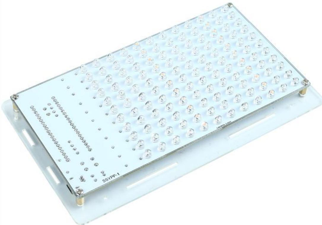
Step 21: Install the 4pcs acrylic panels on the side and fix by 4pcs M2+10mm Screw and 4pcs M2 Nut. Pay attention to the USB interface. Users can use tweezers to clamp the nut and fix the screw when installing M2 screws.
