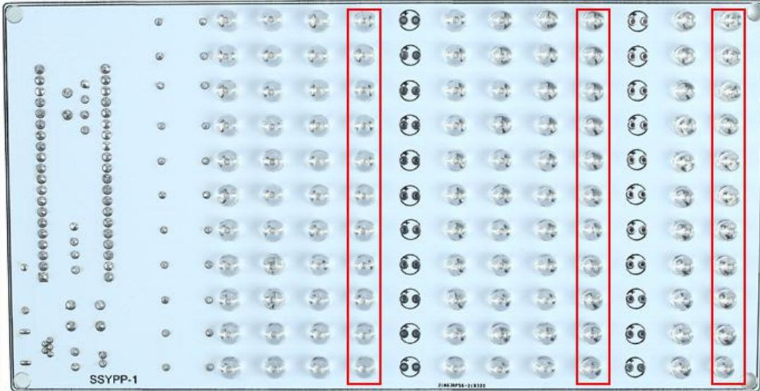
Step 16: Install 22pcs 5mm Pink LED at D45-D55,D100-D110 in the 5th & 10th columns from left as shown.
