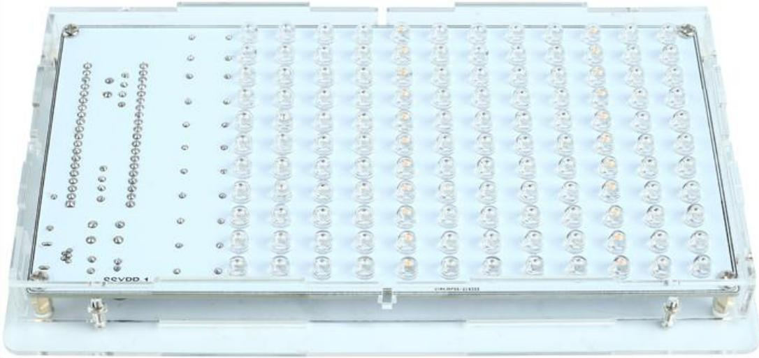
Step 22: Install 1pcs Acrylic board by 4pcs M3+6mm Screw and 4pcs M2+10mm Screw and 4pcs M2 Nut on the top of the PCB.
