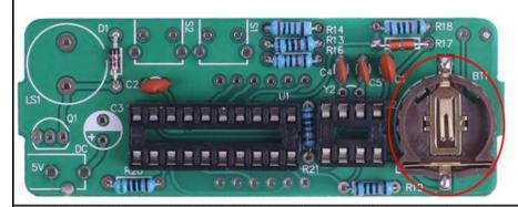
Step 12: Install 1pcs TO-92 S8550 Transistor at Q1.Pay attention to the installation direction of arc.
