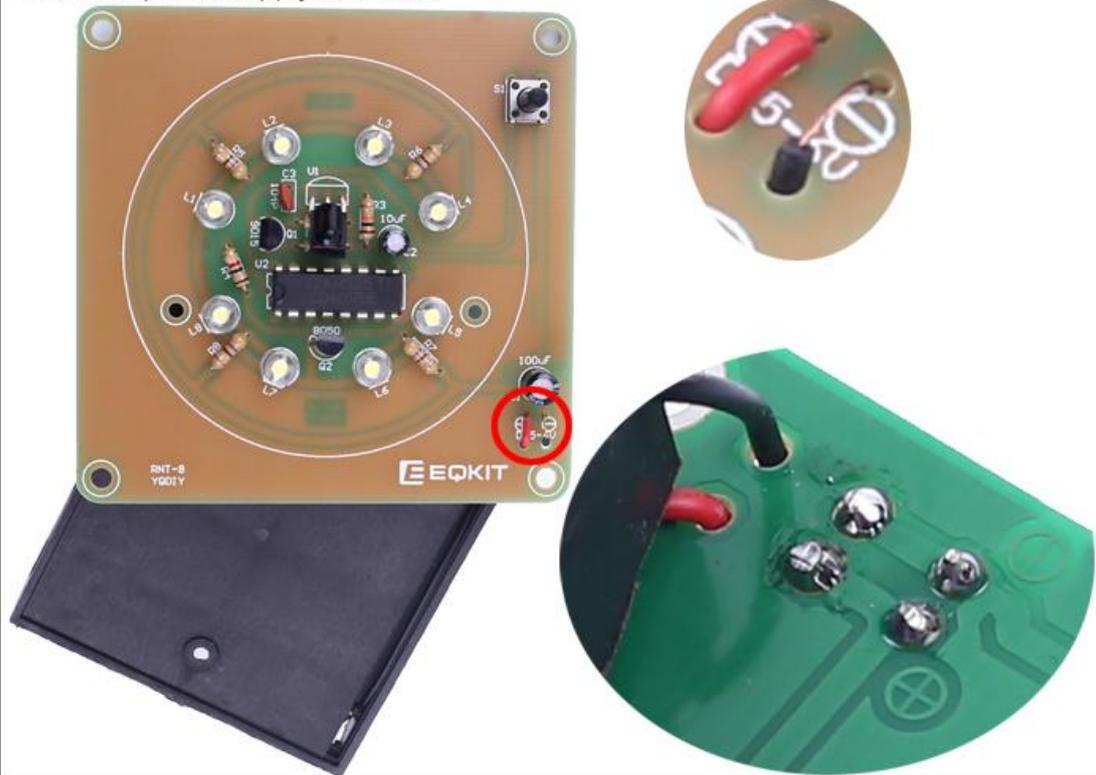
Step 15: Fix battery box by 2pcs M2\*8 Screw and 2pcs M2 Nut if installed battery box.
