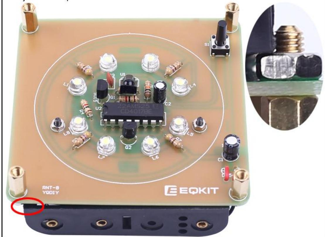
Step 17: Tear off the protective film on the black acrylic surface.
