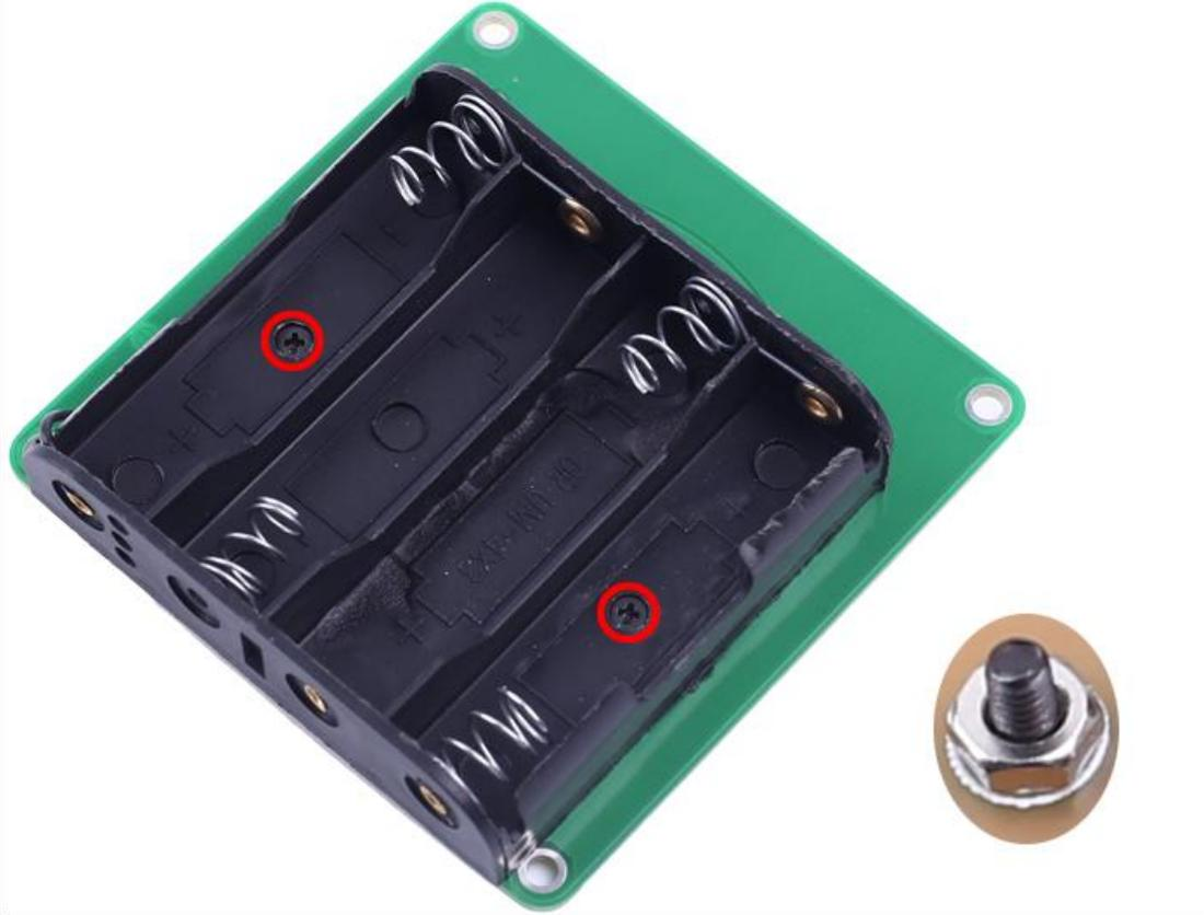
Step 16: Install 4pcs M3\*10+6 Copper Cylinder and 4pcs M3 Nut on PCB. May need to adjust the nut position.
