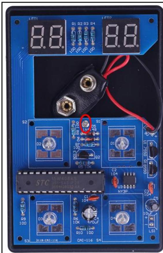
Step 19: Place speaker on case and fix PCB on case by 1pcs 1.7mm Self-tapping screw.
