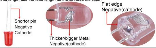
Step 6: Install 3pcs 3mm Green LED at D63,D64,D65. Note: The longer pin connect to square pad.
