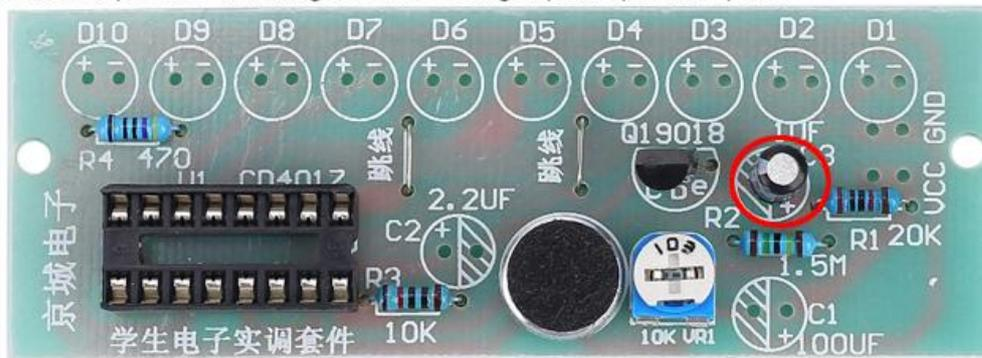
Step 11: Install 1pcs 2.2uF Electrolytic Capacitor at C2. Pay attention to distinguish between positive and negative. The Longer pin is positive pole.
