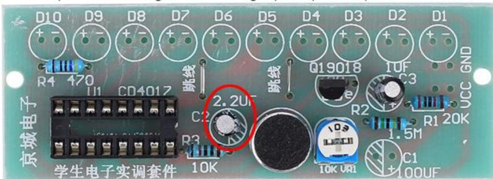
Step 12: Install 1pcs 100uF Electrolytic Capacitor at C1. Pay attention to distinguish between positive and negative. The Longer pin is positive pole.
