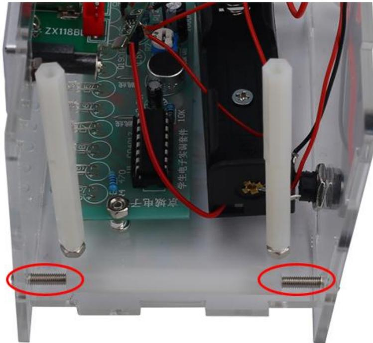
Step 41: Install 2pcs speakers and then fix 4pcs M3\*50mm screws completely.
