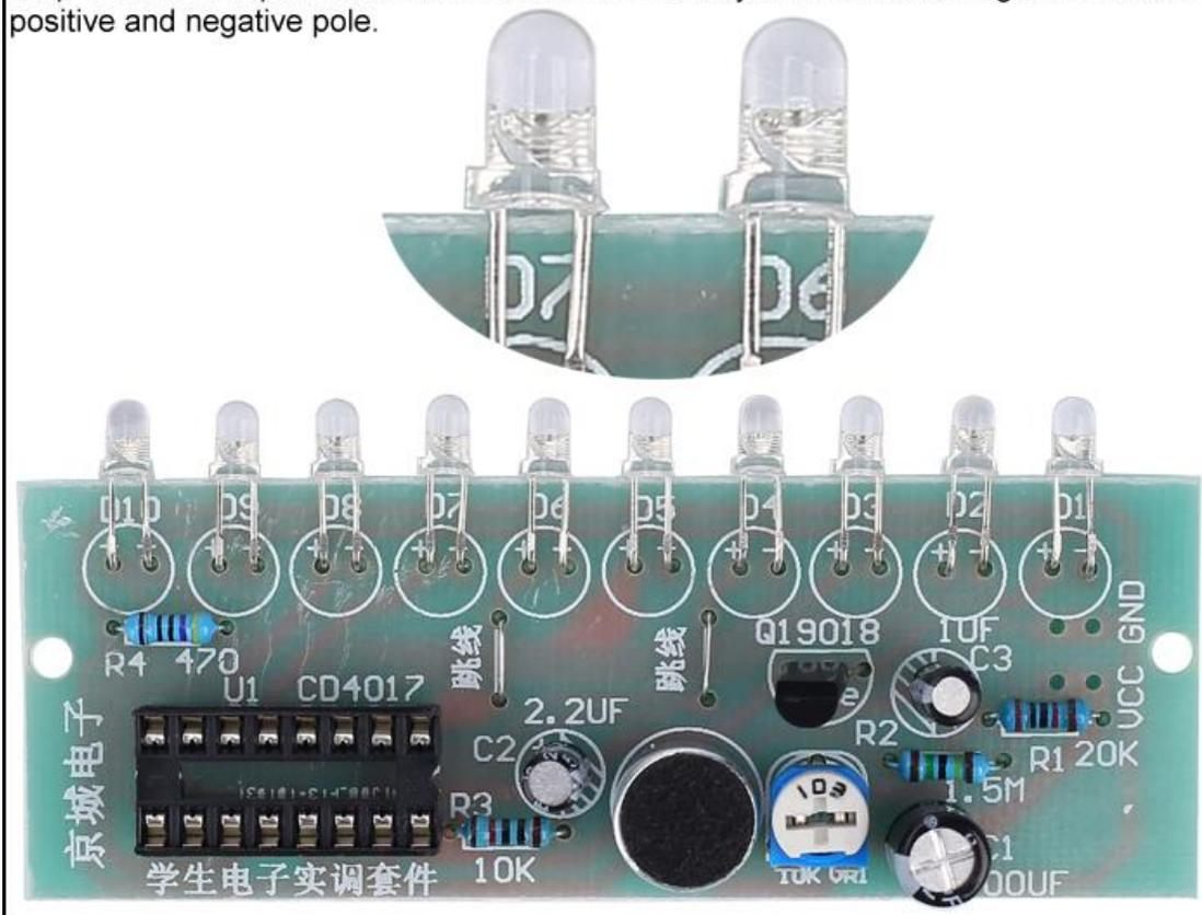
Step 15: Install 1pcs DIP-16 IC CD4017. There is a gap mark on one end of the IC and there is a gap mark on DIP-16 IC Socket where the IC can place on. These two marks are corresponding to each other and are used to specify installation direction of the IC.
