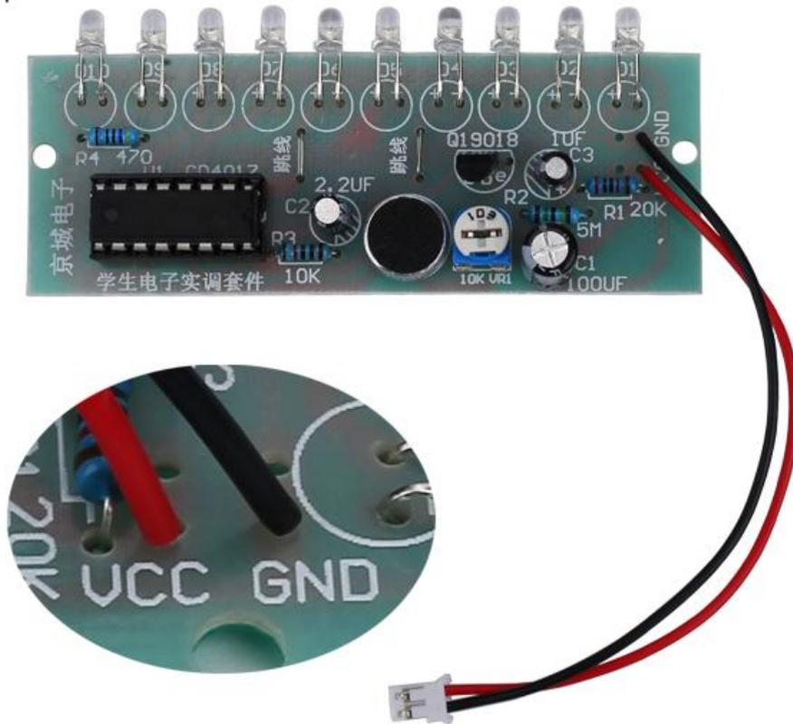
Step 28: Connect 1pcs 15cm Blue or Black Wire to GND pad on LED board.
