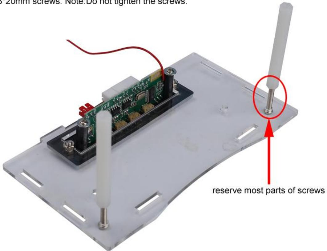
40>.Step 40: Fix Control Acrylic Plate and Socket Acrylic Plate by Nylon Through Column.
