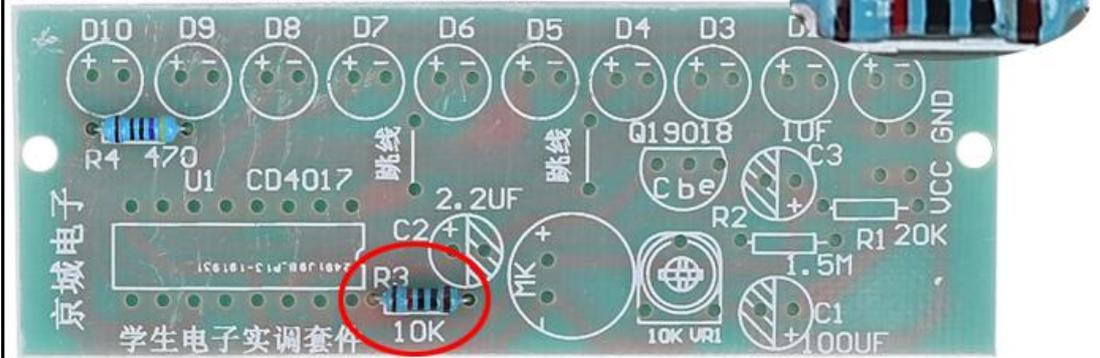
Step 3: Install 1pcs 20Kohm Metal Film Resistor at R1.
