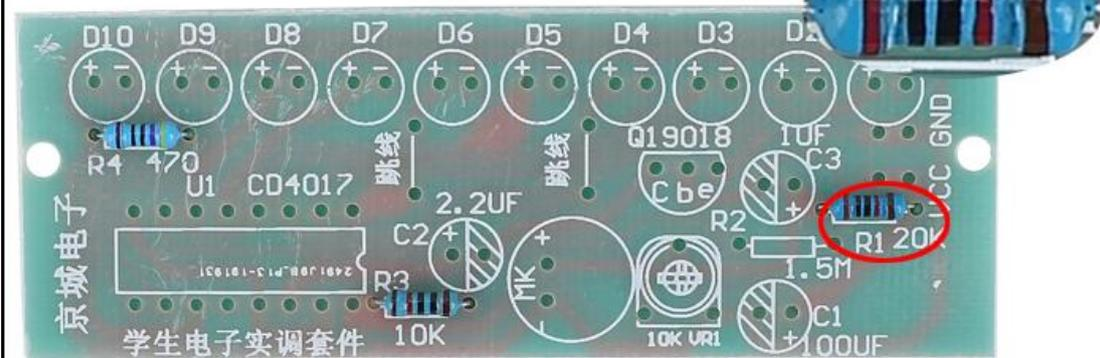
Step 4: Install 1pcs 1.5Mohm Metal Film Resistor at R2.
