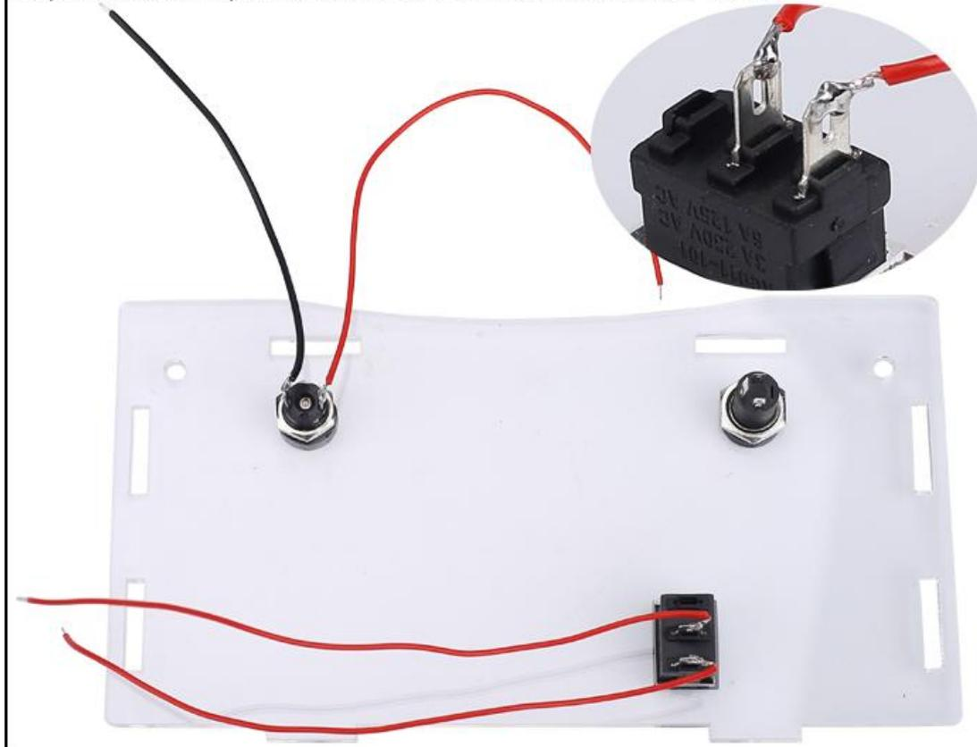
Step 23: Connect 1pcs 30cm Red Wire for Antenna to Antenna Socket.
