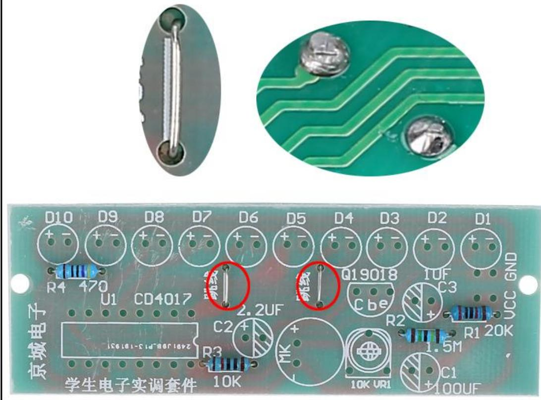
Step 6: Install 1pcs DIP-16 IC Socket at U1. There is a gap mark on one end of the IC Socket and there is a gap mark on PCB silk screen where the IC Socket can place on. These two marks are corresponding to each other and are used to specify the installation direction of the IC Socket.
