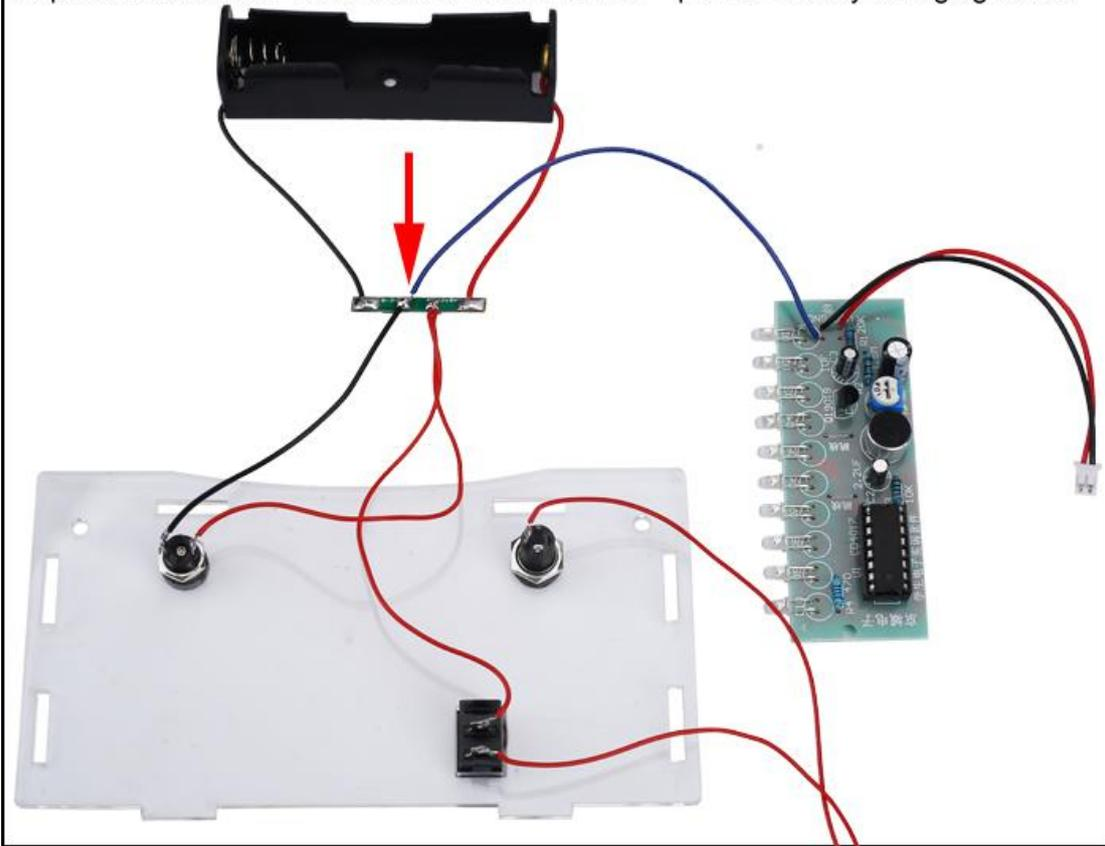
Step 30: Connect another red wire from Power Switch to VCC pad on LED Board.
