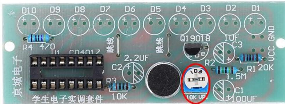
Step 10: Install 1pcs 1uF Electrolytic Capacitor at C3. Pay attention to distinguish between positive and negative. The Longer pin is positive pole.
