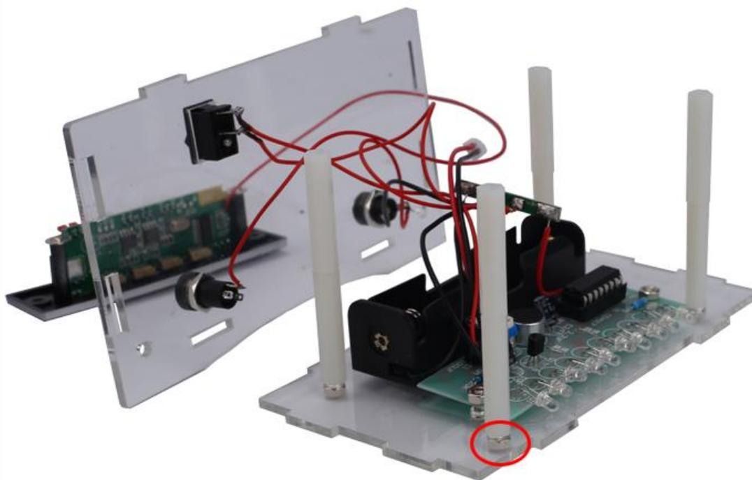
Step 39: Install 2pcs M3\*50mm Nylon Through Column on another acrylic plate by M3\*20mm screws. Note:Do not tighten the screws.
