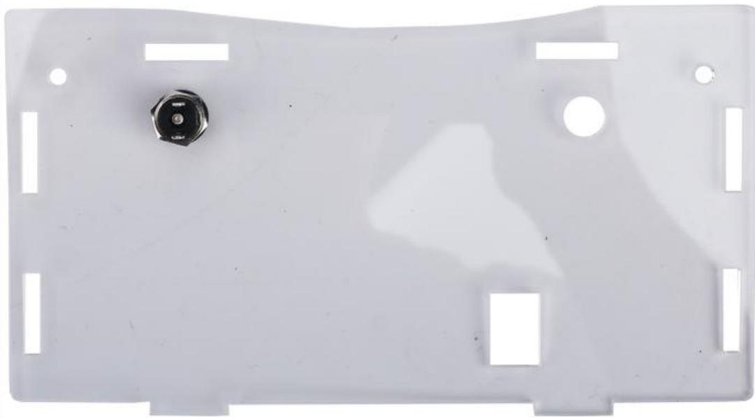
Step 19: Fix 1pcs antenna socket by the biggest nut on acrylic board. Pay attention to the comparison diagram and the front and back of the acrylic.
