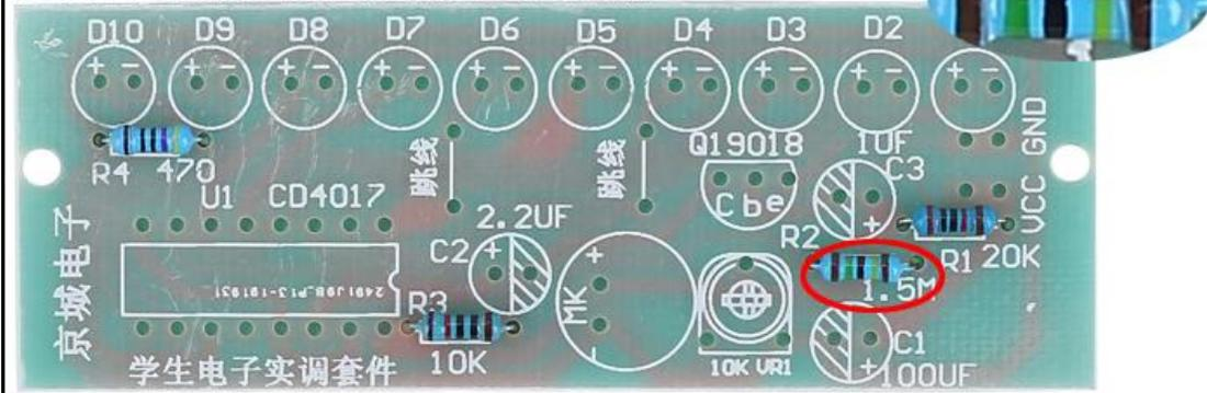
Step 5: Using the resistor pin metal wire that just cut, connect the 2 jumper pads.
