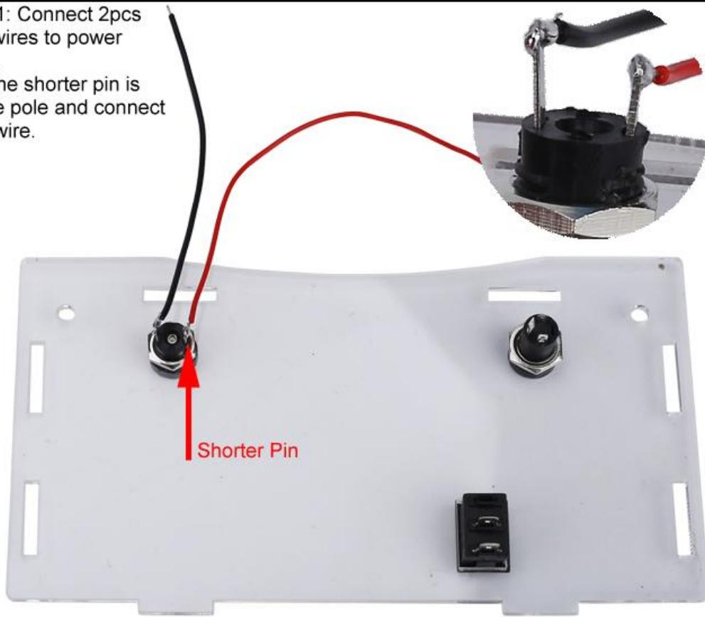
Step 22: Connect 2pcs 20cm Red Thin Wires to Black Power Switch.
