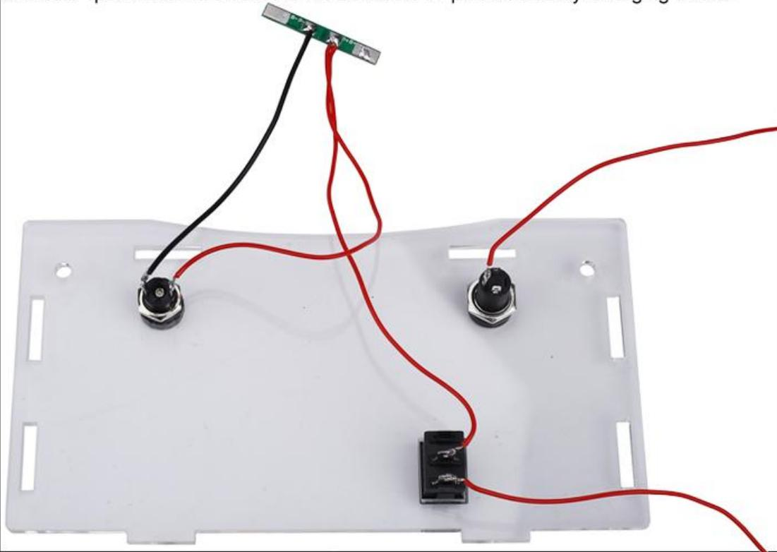
Step 26: Connect red wire form battery box to B+ pad on Battery Charging Board.
