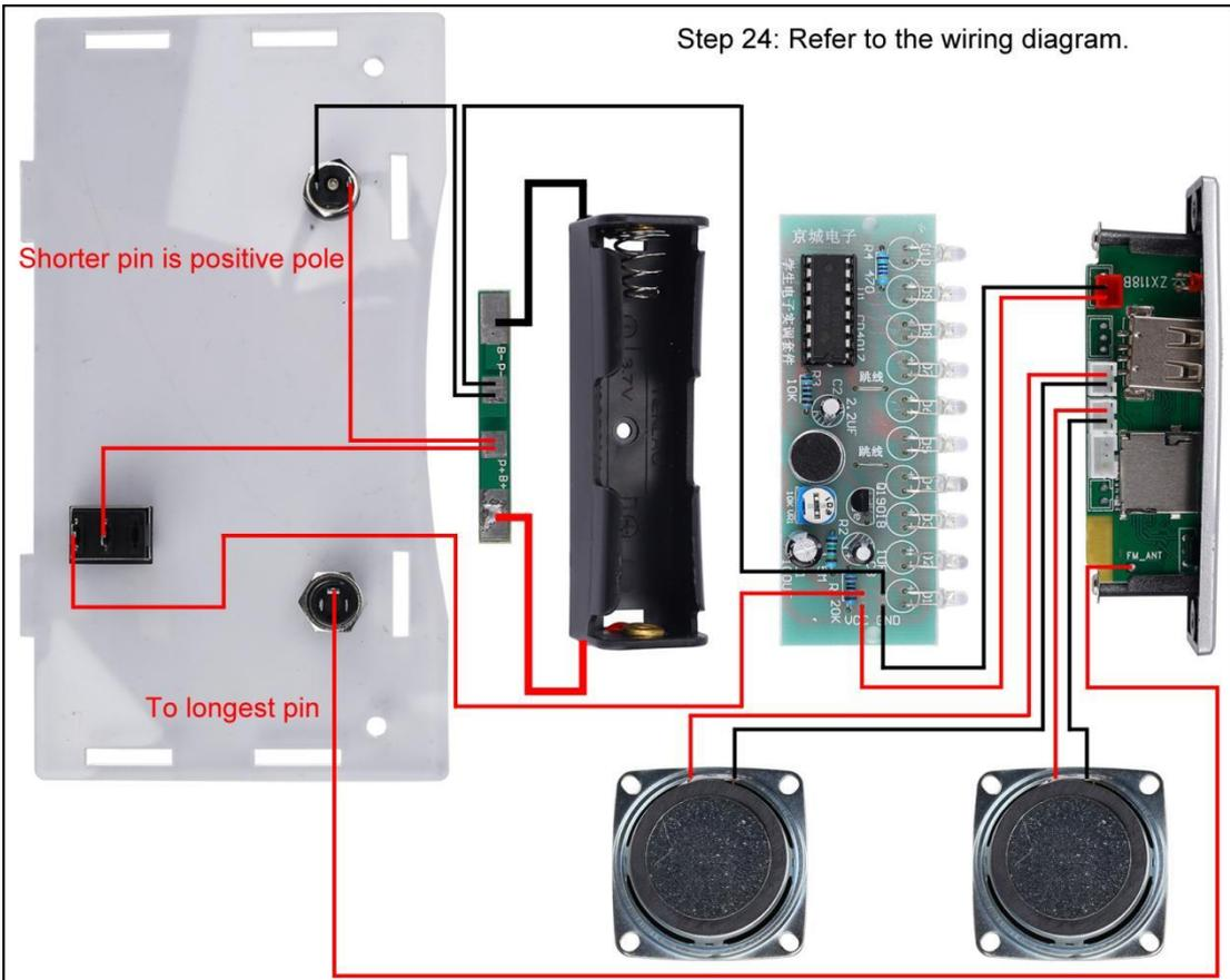
Step 25: Connect 2pcs red wires from Power Socket and Black Power Switch to P+ pad on Battery Charging Protection Board.
