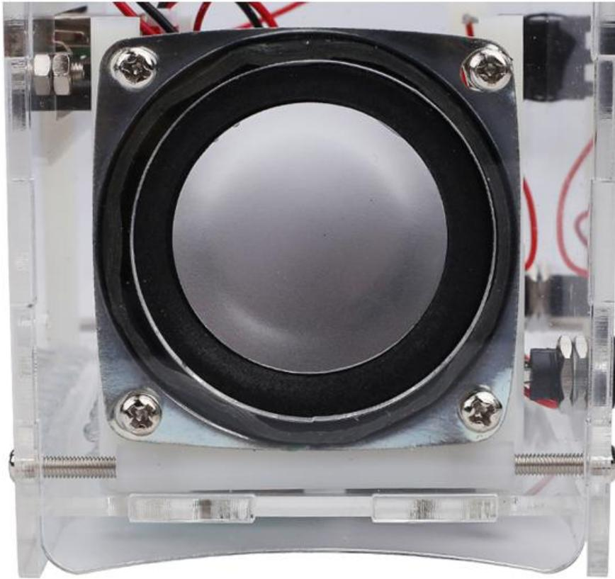
Step 42: Connect power wire from LED board to red socket on Bluetooth controller. Connect speaker to white 2Pin PH2.0 socket. Then install one 18650 rechargeable lithium battery.
