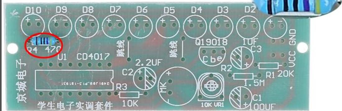
Step 2: Install 1pcs 10Kohm Metal Film Resistor at R3.
