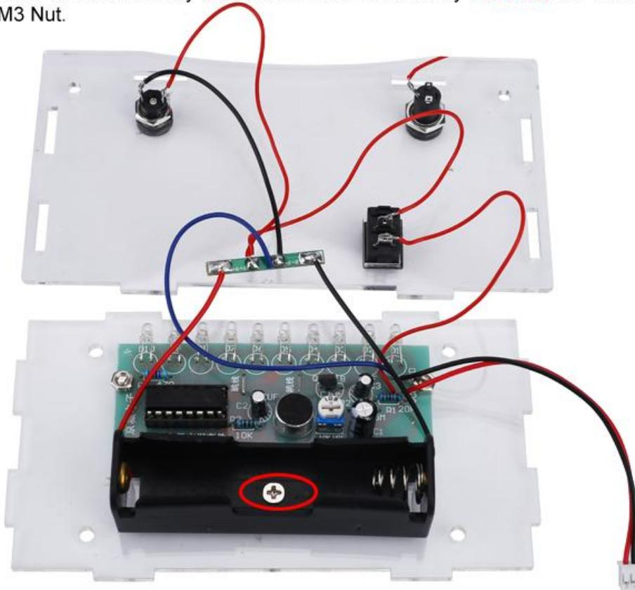
Step 34: Fix Bluetooth audio controller on acrylic panel by 2pcs M3\*8mm Screw and 2pcs M3 Nut.
