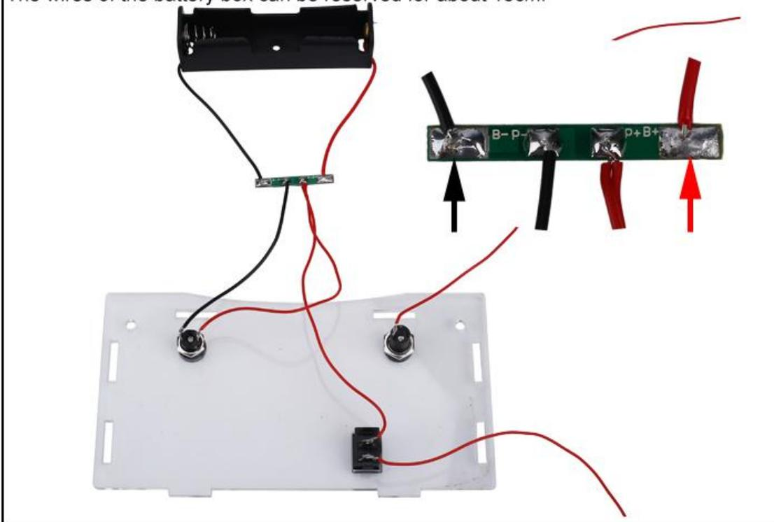
Step 27: Connect 1pcs 10cm 2Pin PH2.0 Wire on LED board. Red wire connect to VCC pad.
