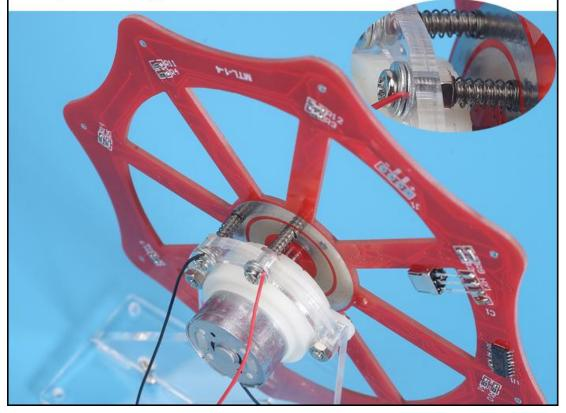
Step 17: Fix PCB on motor shaft by 1pcs Acrylic PCB Fix Bracket, 1pcs M3 Pad, 1pcs M3 Nut.
