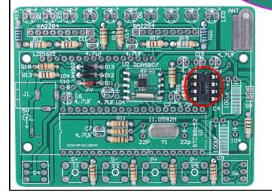
Step 14: Install 1pcs DIP-40 IC Socket at U1. There is a gap mark on one end of the IC Socket and there is a gap mark on PCB silk screen where the IC Socket can place on. These two marks are corresponding to each other and are used to specify the installation direction of the IC Socket.
