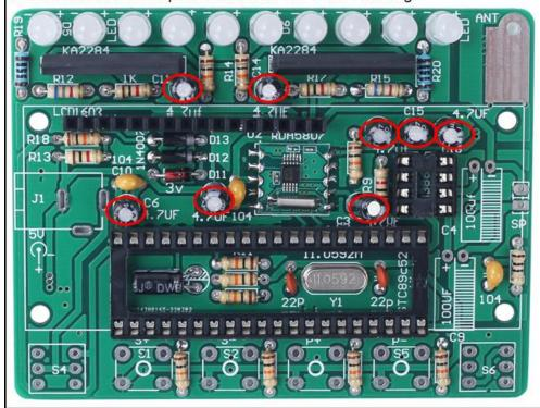
Step 25: Install 2pcs 100uF Electrolytic Capacitor at C4,C9.Pay attention to distinguish between positive and negative.The Longer pin is positive pole. Note: The capacitor needs to be placed horizontally, keep a distance of 2mm between the capacitor and the PCB when installing.
