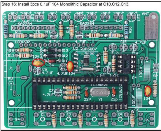
Step 17: Confirm and identify the installation direction of the KA2284.
