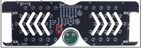
Step 5: Identify the positive(anode) and negative(cathode) lead of LED. The leads of the LED must be installed correctly, otherwise the LED cannot be turned on. Here are four methods as following:
