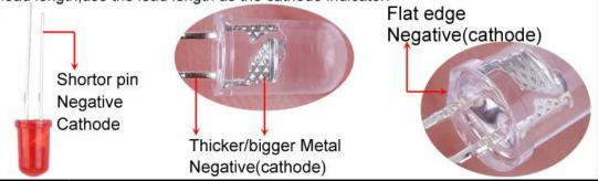
Step 6: Install 50pcs 3mm LED at D1-D50. Pay attention to distinguish between positive and negative pole.
