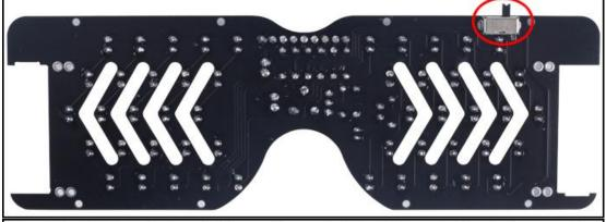
Step 13: Install 2pcs battery holder positive metal sheet. Pay attention to placement.
