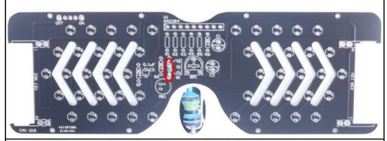
Step 2: Install 3pcs 10Kohm Metal Film Resistor at R6,R7,R9.
