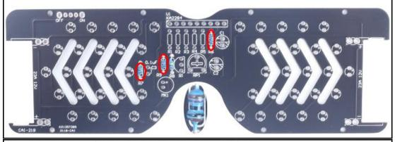
Step 3: Install 5pcs 1Kohm Metal Film Resistor at R1-R5.
