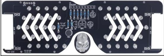
Step 7: Install 1pcs 0.1uF 104 Ceramic Capacitor at C3.
