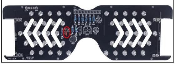
Step 8: Install 1pcs ZIP-9 KA2284 LED Driver at U1. Pay attention to the mounting direction as showing. 00 Step 9: Install 1pcs TO-92 S9014 Transistor at Q1. Pay attention to the mounting direction as showing. 00000 Step 10: Install 2pcs 10uF Electrolytic Capacitor at C1,C2.Pay attention to distinguish between positive and negative. The Longer pin is positive pole. 00000
