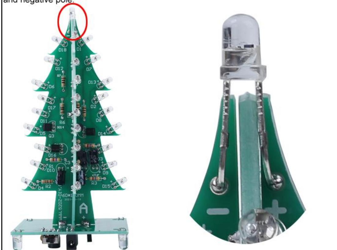
Step 17: Test. Connect 5V USB power supply to test LED. It is OK if all LED flash automatically after turning on the power switch.
