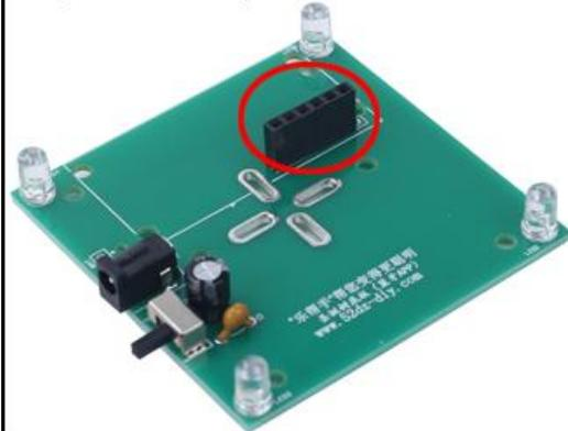
Step 14: Splicing PCB-A and PCB-B, pay attention to align the fixing points, and then fix it with solder wire. Pay attention to the splicing direction.
