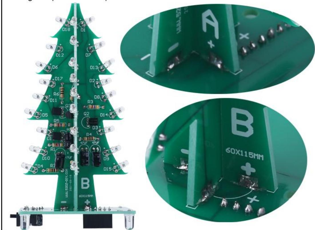
Step 16: Install 1pcs 3mm RGB LED at top. Pay attention to the direction of positive and negative pole.
