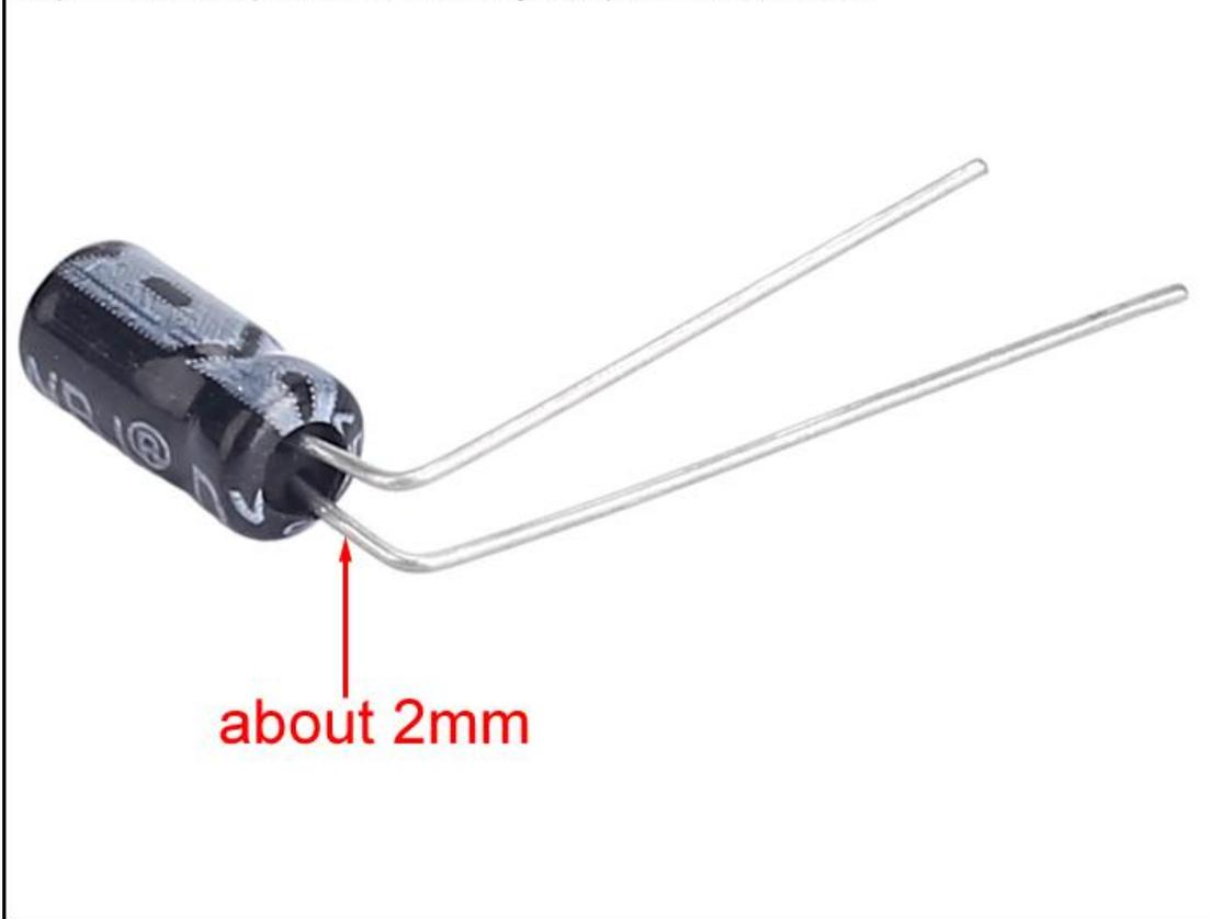
Step 7: Install 6pcs 47uF Electrolytic Capacitor at C1,C2,C3 on PCB-A/B.
