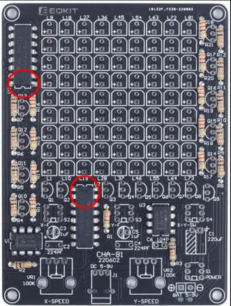
Step 6: Install 1pcs 0.1uF 104 Ceramic Capacitor at C6.
