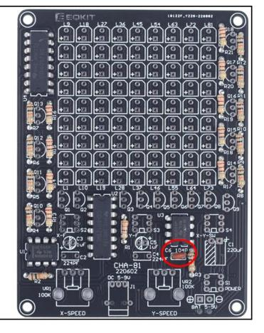
Step 7: Install 1pcs 0.22uF 224 Ceramic Capacitor at C2,C4.
