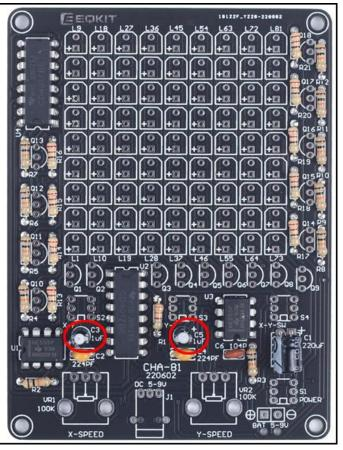
Step 10: Install 18pcs TO-92 S9014 Transistor at Q1-Q18. Pay attention to the installation direction.
