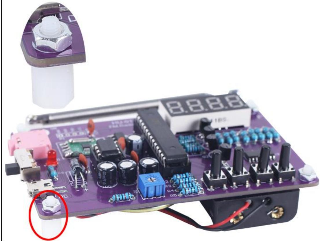
Step 31: Tear off the protective film on the surface of the acrylic shell.
