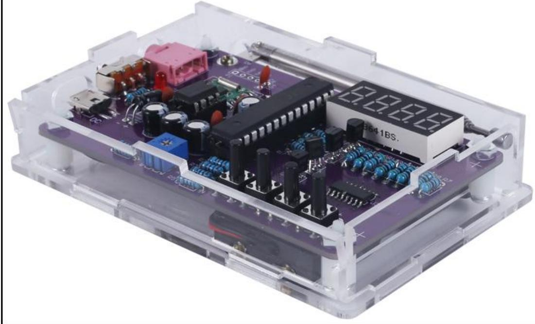
Step 34: Fix Top Acrylic Board by 4pcs M2\*22mm Screw and 4pcs M2 Nut.
