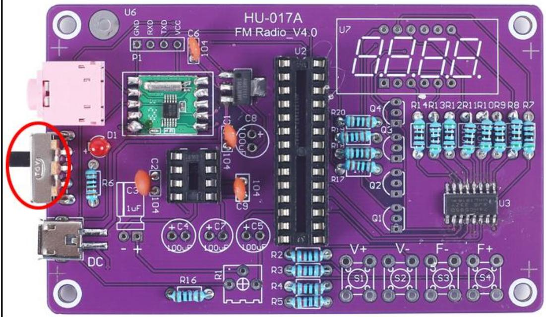
Step 17: Install 4pcs 100uF 16V Electrolytic Capacitor at C4,C5,C7,C8. Pay attention to distinguish between positive and negative. The Longer pin is positive pole.
