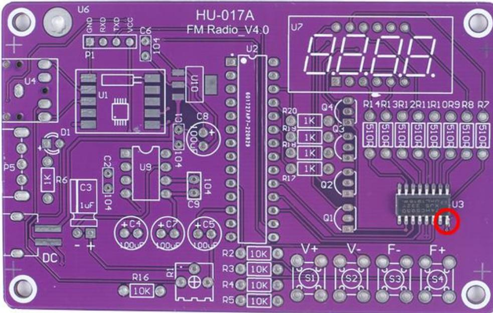
**Step 4: Connect others pads on 74HC595D to pads on PCB by tin and soldering iron.**
