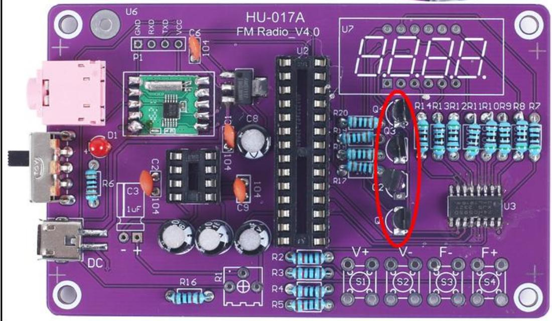
Step 19: Install 1pcs 4Bit Red Digital Tube at U7.
