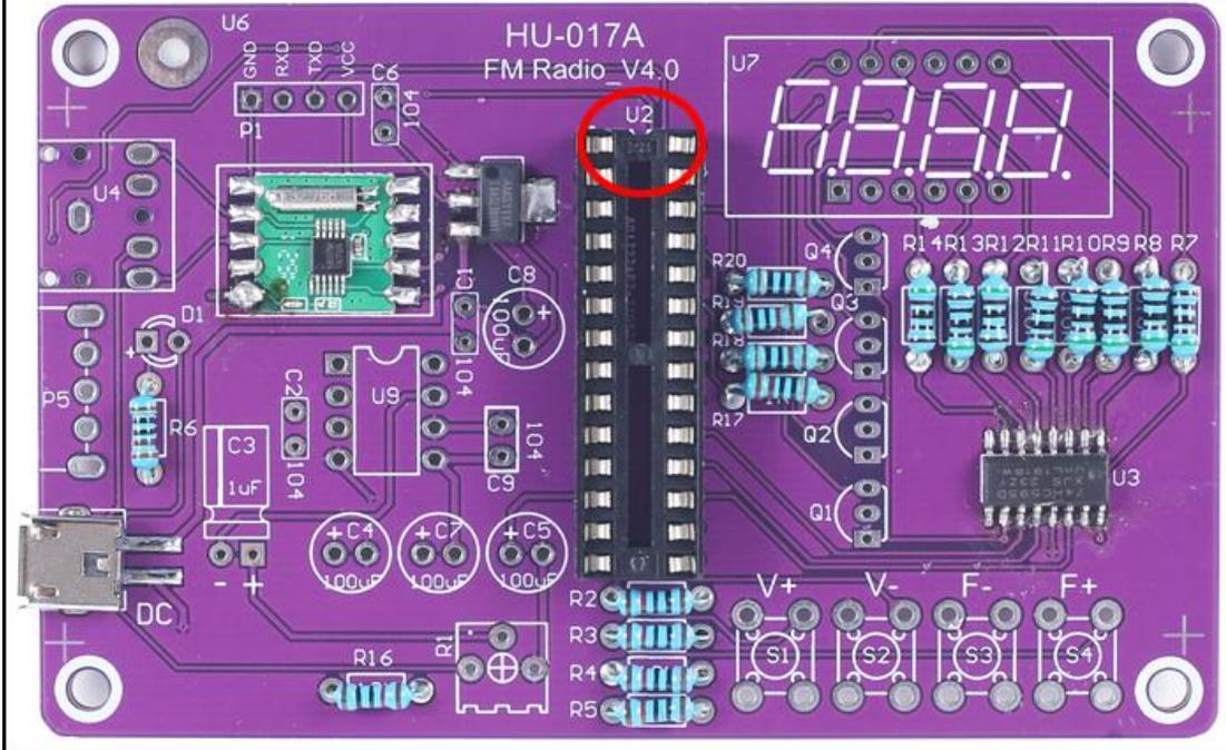
Step 12: Install 1pcs DIP-8 IC Socket at U9. There is a gap mark on one end of the IC Socket and there is a gap mark on PCB silk screen where the IC Socket can place on. These two marks are corresponding to each other and are used to specify the installation direction of the IC Socket.
