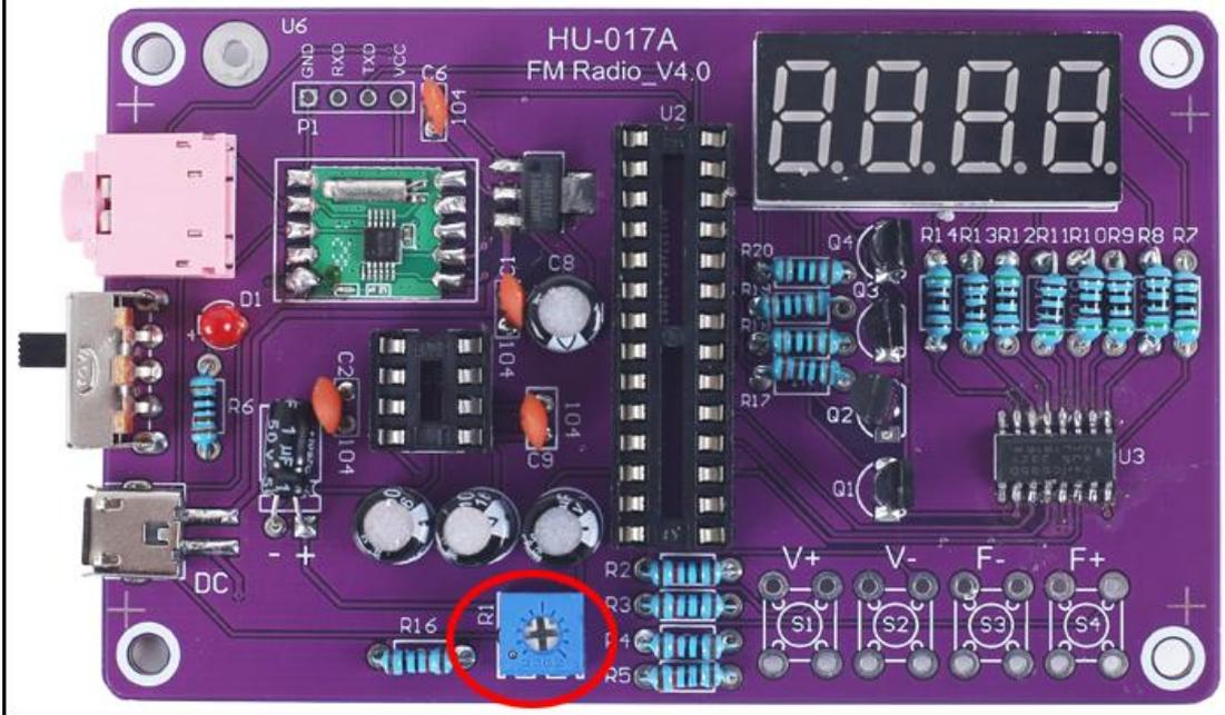
Step 22: Install 4pcs 6\*6\*8mm Black Button at S1-S4. Ensure that the buttons are installed vertically to avoid affecting the next installation of acrylic plates.
