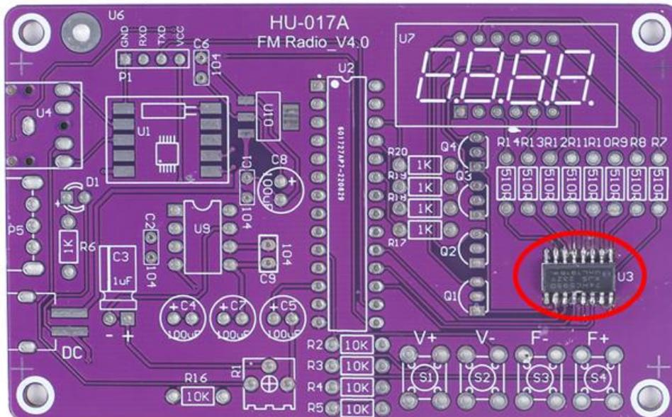
Step 5: Install 1pcs SOT-223 AMS1117-3.3V Voltage Converter at U10 by the same method.
