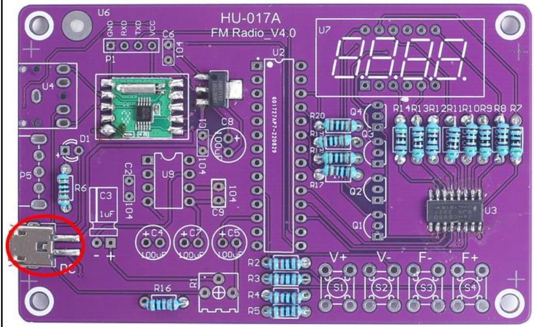
Step 11: Install 1pcs DIP-28 IC Socket at U2. There is a gap mark on one end of the IC Socket and there is a gap mark on PCB silk screen where the IC Socket can place on. These two marks are corresponding to each other and are used to specify the installation direction of the IC Socket.
