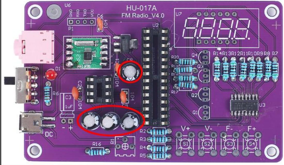
Step 18: Install 1pcs TO-92 S8550 Transistor at Q1-Q4. Pay attention to the installation direction. The arc on the PCB corresponds to the arc of the components.
