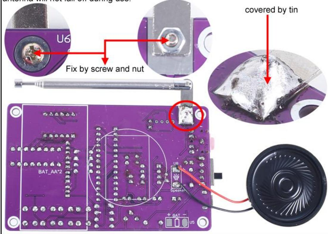
Step 28: Connect AA\*2 battery box to PCB. Red wire to '+' pad.
