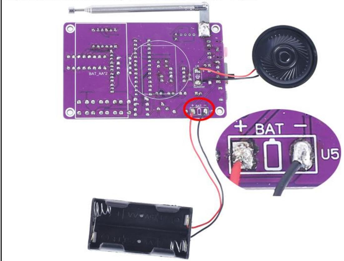
Step 29: Paste the speaker and battery box on the PCB back with double-sided adhesive tape, and pay attention to the white line area on the PCB to define their positions.
