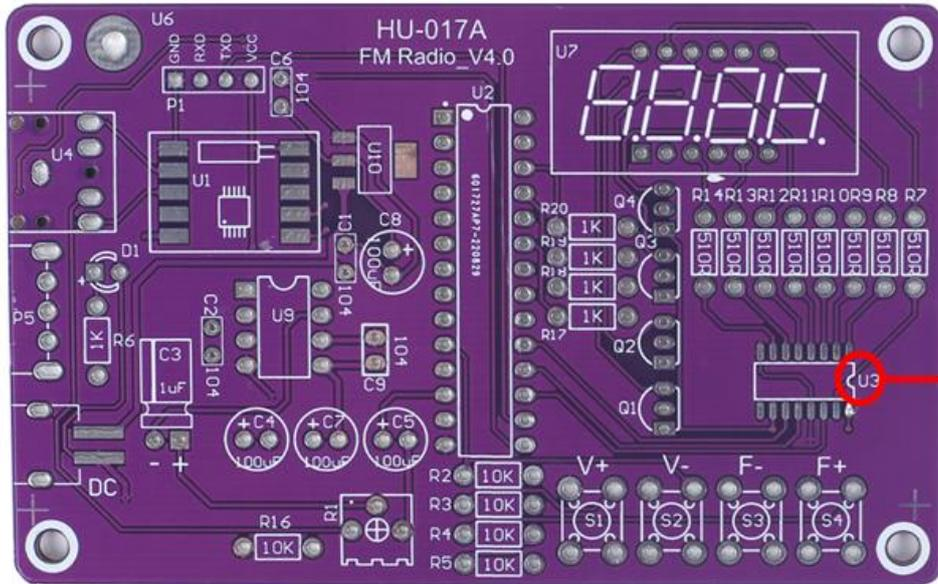
Step 2: Randomly choose a pad on the PCB, and then melt the solder on this pad.
