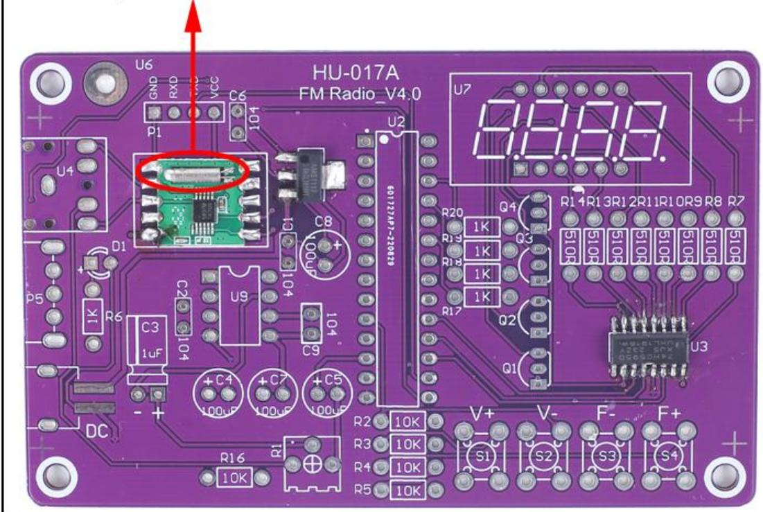
Step 7: Install 8pcs 510ohm Metal Film Resistor at R7-R14.
