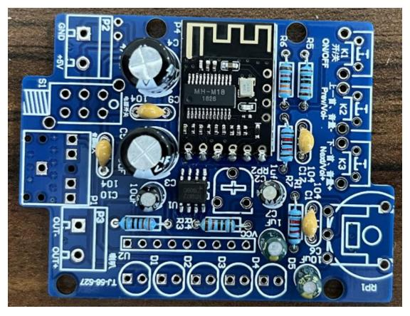
Step 6: Install blue and white adjustable resistors.
