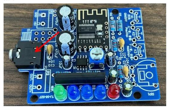
Step 10: Install the Dial Potentiometer.
