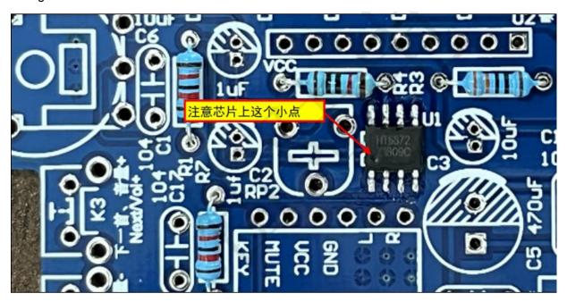
**Step 3: Install Ceramic/monolithic capacitors.**
