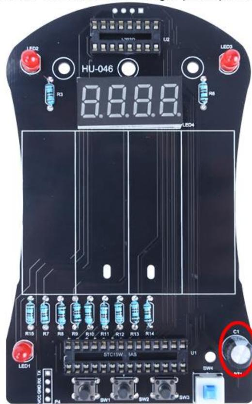
Step 9: Install 1pcs DIP-28 IC STC15W408AS Controller. There is a gap mark on one end of the IC and there is a gap mark on DIP-28 IC Socket where the IC can place on. These two marks are corresponding to each other and are used to specify the installation direction of the IC.
