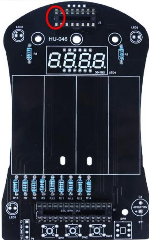
Step 4: Install 3pcs 5mm Red LED at LED1-LED3. Note: The longer pin is positive pole and connect to '+' pads.
