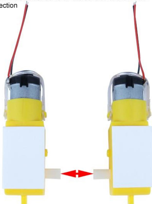
Step 14: Paste 2pcs motors onto the surface of the PCB. Note: The motor should be as close to the edge of the PCB as possible to avoid affecting the installation of the wheels and causing them to get stuck by the PCB.
