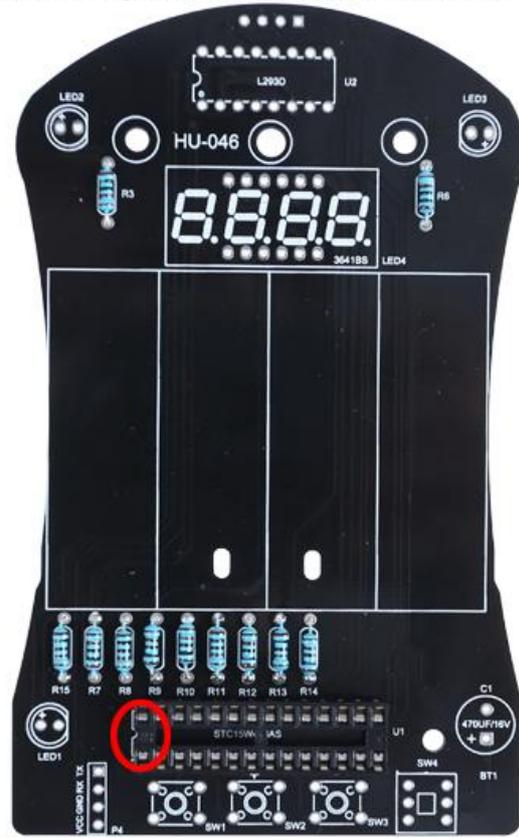
Step 3: Install 1pcs DIP-28 IC Socket at U2 in the same methods.
