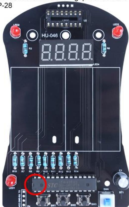
Step 10: Install 1pcs DIP-16 IC L293D Motor Driver at U2 in the same methods.
