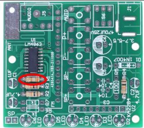
Step 7: Install 2pcs 1Kohm Metal Film Resistor at R6,R7.
