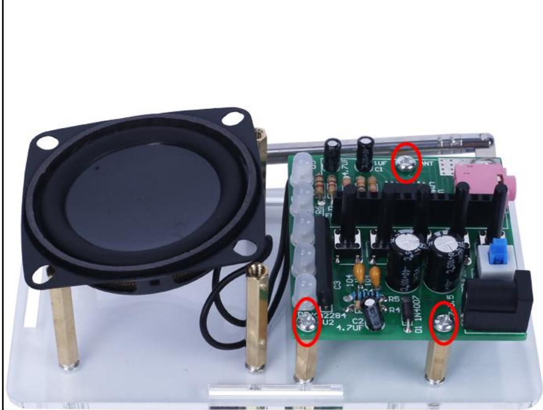
Step 28: Install TOP acrylic plate and note the antenna mounting hole and direction.
