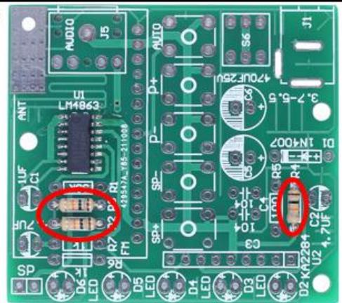
Step 6: Install 1pcs 39Kohm Metal Film Resistor at R1.
