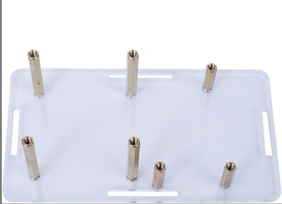
Step 27: Fix PCB on 3pcs M3\*15mm Copper Pillar by 3pcs M3\*6mm Screw.
