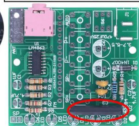
Step 13: Install 5pcs 5mm RGB LED at D2,D3, D4,D5,D6. Note:The longer pin is positive pole and connect to ' + ' pads.
