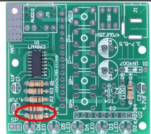
Step 8 Install 1pcs 100ohm Metal Film Resistor at R5.
