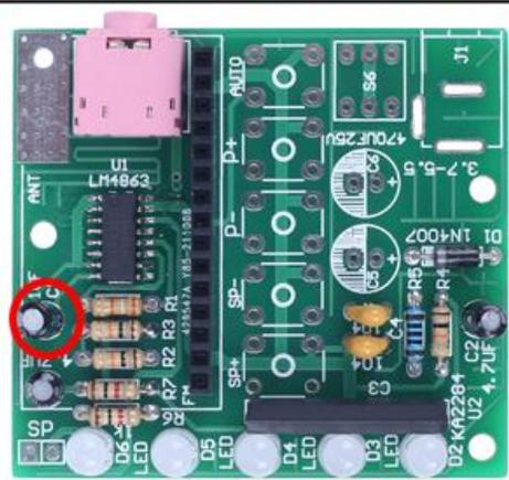
Step 17: Install 2pcs 470uF Electrolytic Capacitor at C5,C6. Pay attention to distinguish between positive and negative. The Longer pin is positive pole.
