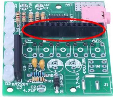
Step 15: Install 2pcs 4.7uF Electrolytic Capacitor at C2,C7. Pay attention to distinguish between positive and negative. The Longer pin is positive pole.
