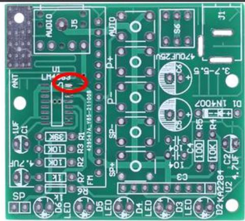
Step 3: Fix LM4863: Use a soldering iron to melt tin on the pad just now and hold LM4863 with tweezers in the other hand to place/press on U1 to prevent movement. Take care to match and align each pads. Then remove soldering iron. Then remove tweezers after solder tin cooling and solidification.
