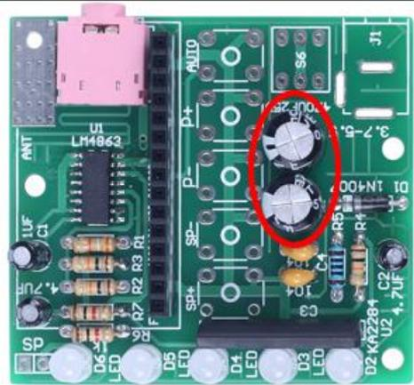
Step 18: Install 1pcs 8\*8mm Self-locking Button at S6.
