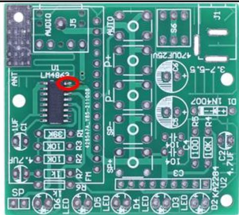
Step 4: Connect others pads on LM4863 to pads on PCB by tin and soldering iron
