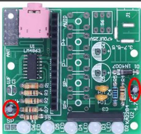
Step 16: Install 1pcs 1uF Electrolytic Capacitor at C1. Pay attention to distinguish between positive and negative. The Longer pin is positive pole.
