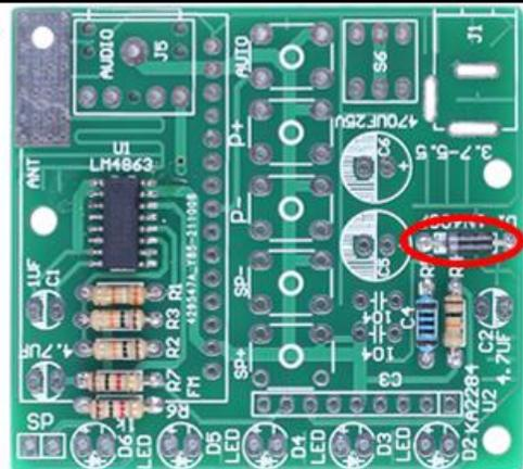
Step 10: Install 2pcs 0.1uF 104 Monolithic Capacitor at C3,C4.
