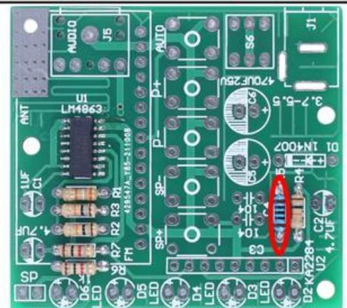
Step 9: Install 1pcs DO-41 1N4007 Diode at D1. Pay attention to the installation direction. There is a white mark on 1N4007 and a white mark on PCB which are used to confirm the installation direction.
