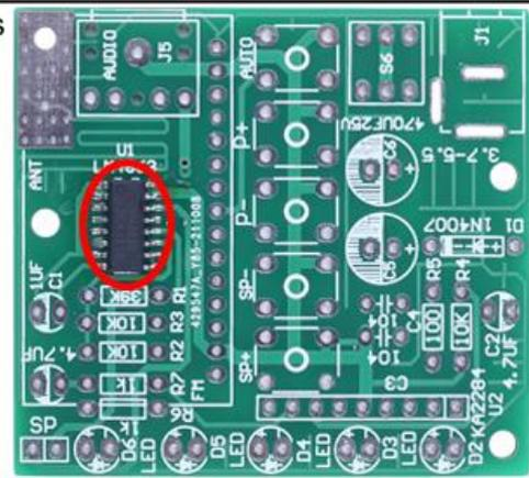
Step 5: Install 3pcs 10Kohm Metal Film Resistor at R2,R3,R4.
