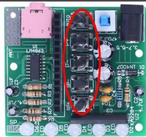
Step 21: Install 1pcs FM Audio Receiver on Female Socket.
