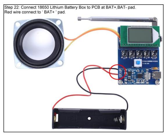
Step 23: Test. Correctly install a rechargeable 18650 battery and test its functions by following 'Use Methods'. Pay attention to the positive and negative poles of the battery otherwise it may damage the circuit board.
