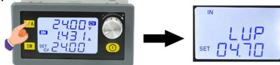
3.1>.At Normal Display Status, keep press **SW** button 2second enter into parameter set interface.
