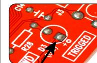
Solder positive pole (the longer lead) to the square pad
