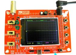
"Trigger" LED blinking twice indicates booting-up is good.
